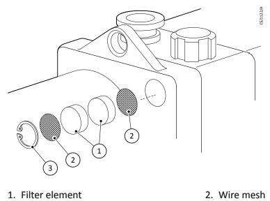
3. Retainer circlip
