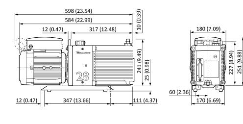
Figure 2 Single-phase motors: Dimensions mm (inches)
