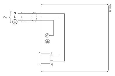
Figure 5 Single-phase motors: 100 V 50 Hz, 100-105 V 60 Hz and 115 V 60 Hz
