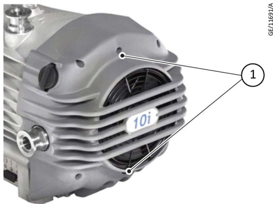
Figure 2 Fan cowl removal
