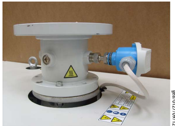
Figure 87 - Installation of the temperature transmitter to the pump inlet spool
